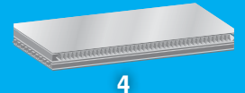
4 BUILD & STACK CORE LAYERS Repeat sequence until core height is achieved, metal band core
